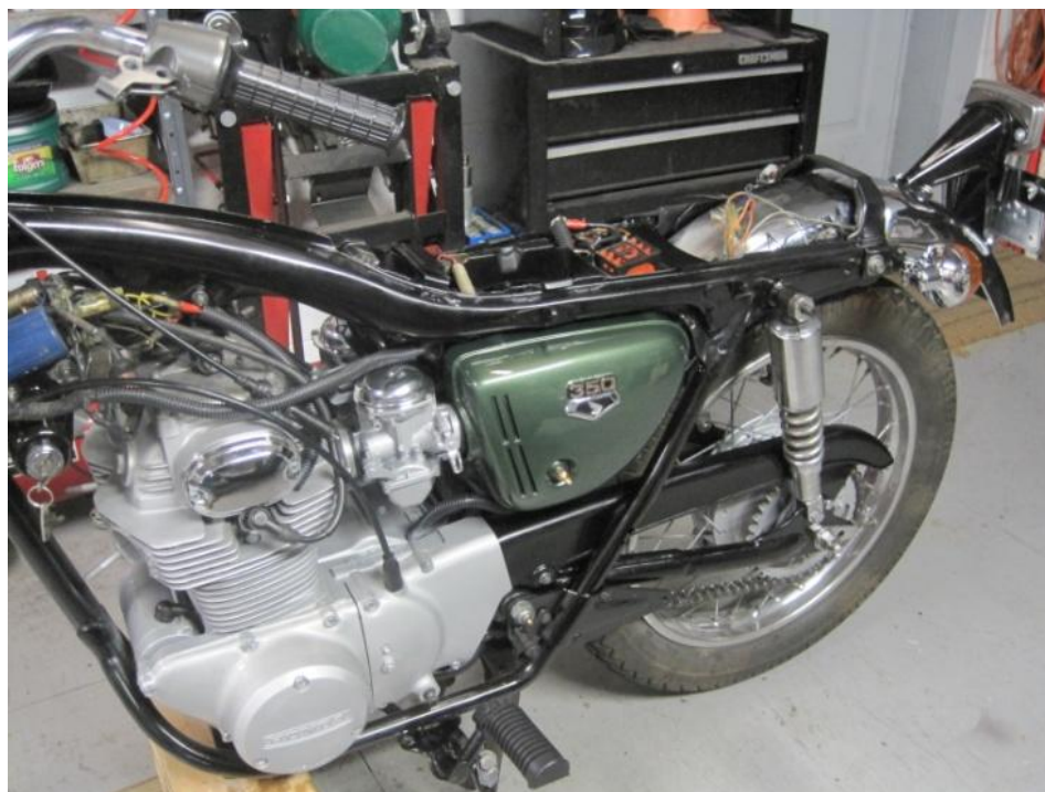
Side cover mounted to the air filter element case.
