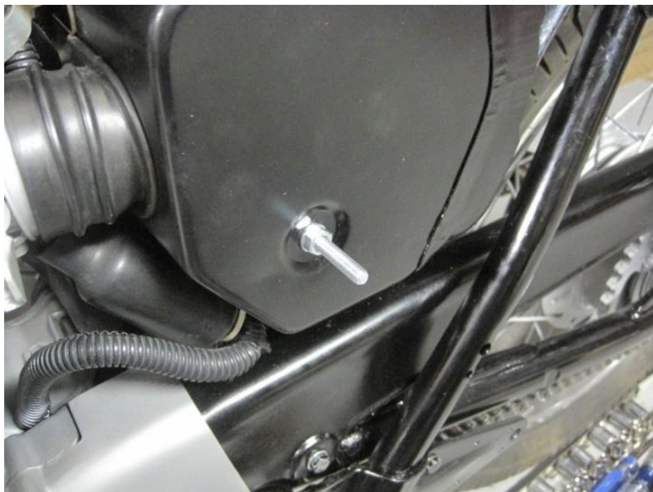
Air filter element and case with mounting bolt.
